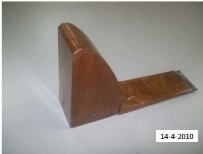
Fig. 6 : Dam Spillway with sloping apron
