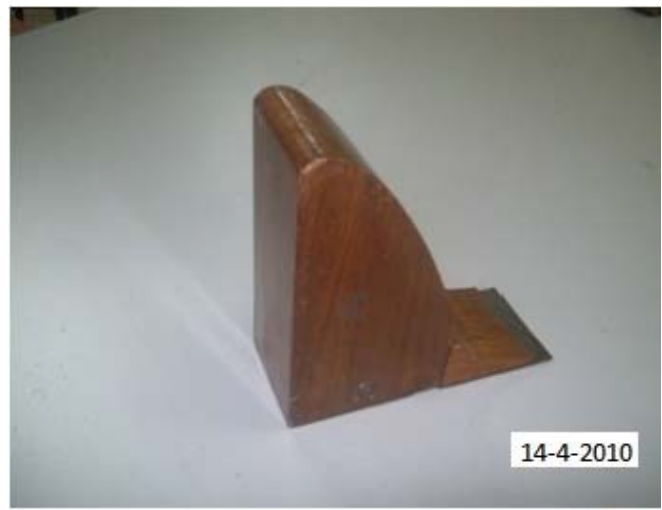
Fig.7 : Dam Spillway with apron blended reverse curvature
