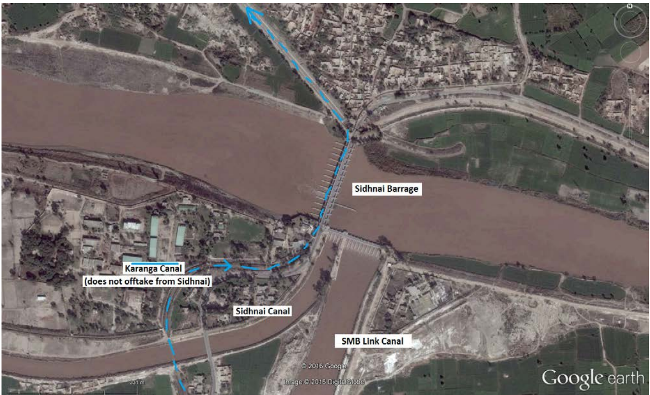
Figure 43 Sidhnaï Barrage showing main barrage and offtake canals
